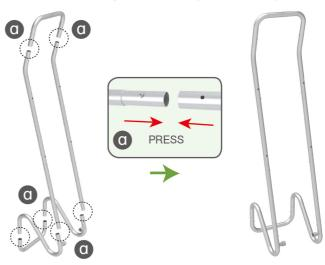
STEP 03 To install the cross bar according to labellings
