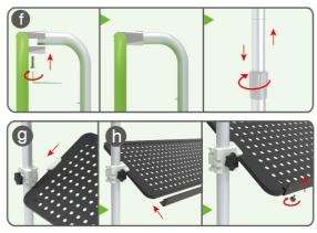
Clip into hanging boards based on directions of three-way clips & tightening with thumb screws, clip F-shaped bar onto hanging board with thumb screws.
